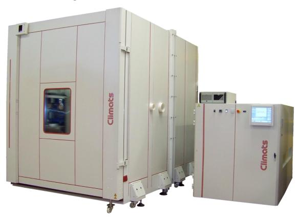
Hot – Cold – Humid climatic chamber of a volume of 13750 dm<sup>3</sup>, meant, among others, to carry out the standards :
