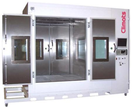
2700 dm<sup>3</sup> one-piece environmental chamber intended for tests in laminar flow atmosphere, within a temperature range from +20°C to +60°C, with air speed rates inside the volume between 0,3 and 0,5 m/s during plateau.
