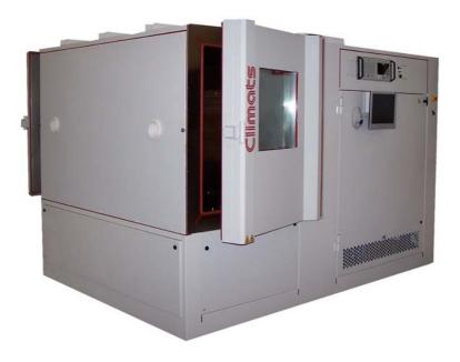
1600 dm<sup>3</sup> one-piece chamber meant to receive large products, long and cylindrical, set on cart.
