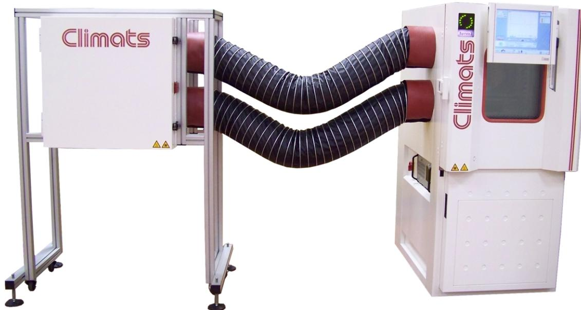
This chamber, from our standard range Excal (8 volumes from 140 to 1800 dm<sup>3</sup>), is transformed into an air generator supplying a recipient cabinet, also made by Climats.
